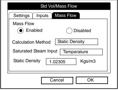
Figure 4-9: The Mass Flow Tab in the Standard Volume/ Mass Flow Option
